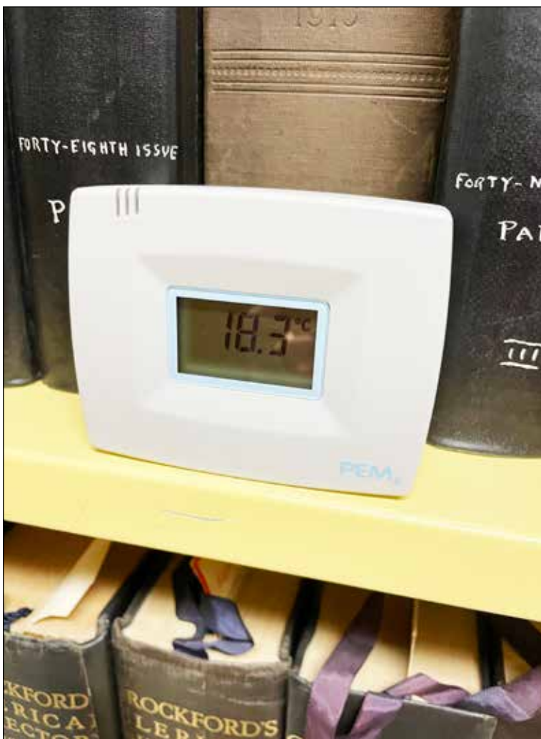
Device monitors the temperature in the vault, which is climate-controlled and has a fire suppression system. These measures slow down deterioration, as the registers are kept at an optimal, consistent temperature and humidity.
